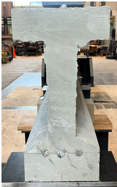
Figure 7: Prestressed beam cross-section
